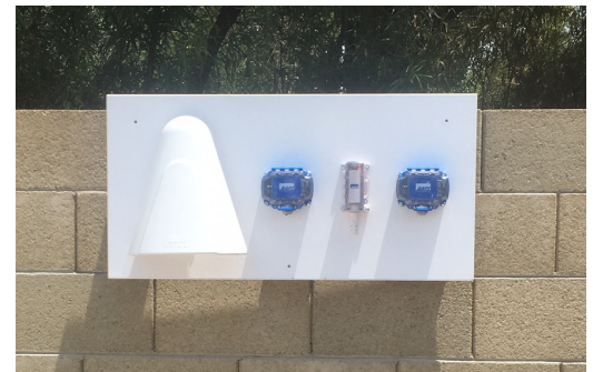
Fig. 2: Sensor mounting with and without Weather Shade in Phoenix, Arizona
