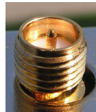
Figure 2: Female RP-SMA (RP-SMA-F or RSMA-F) socket connector: Inner pin contact with a female connector body and outside threads. (Receiver jack)
