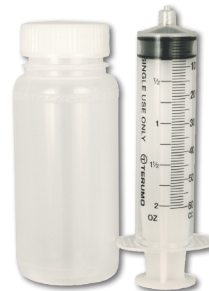
VOC Sensor Verification Kit
