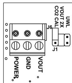
Fig. 6: J1 Set for 0 to 10 VDC Output
