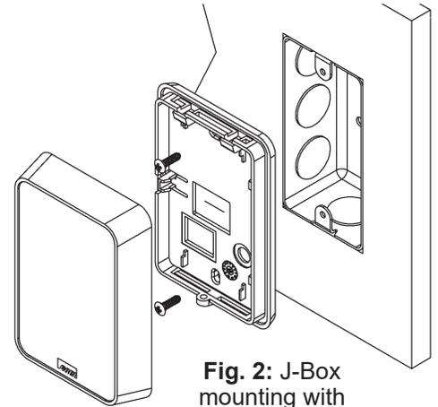
Fig. 2: J-Box mounting with standard base
