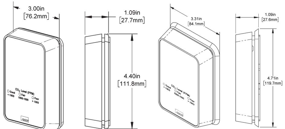
**Fig. 1:** BAPI-Stat “Quantum” CO<sub>2</sub> Sensor (standard mounting base at left and 60mm mounting base for European wall boxes with 60mm mounting centers at right)
