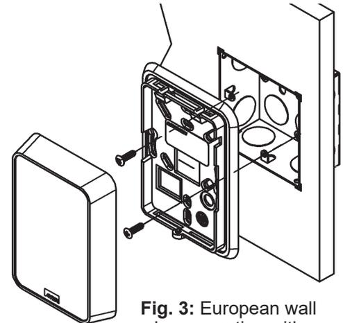
Fig. 3: European wall box mounting with 60mm base
