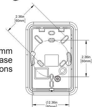
**Fig. 4:** 60mm mounting base dimensions
