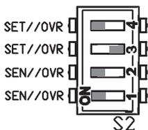
Override in Parallel with Sensor: Common Ground Units
