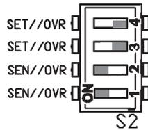
Override in Parallel with Sensor: Differential Ground Units
