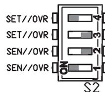
Override as a Separate Output or No Override: Common Ground Units
