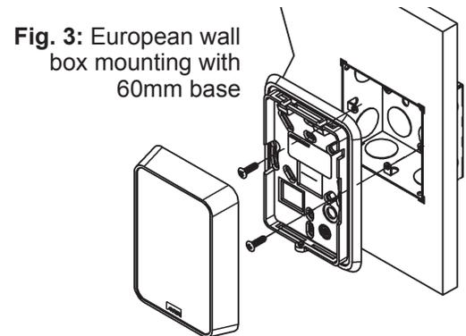
**Fig. 3:** European wall box mounting with 60mm base
