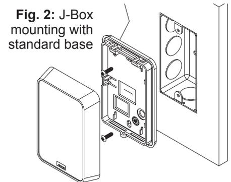
**Fig. 2:** J-Box mounting with standard base
