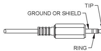
Fig. 8: C35 Comm. Jack (3.5mm plug shown for clarity)
