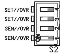
Override as a Separate Output or No Override: Differential Ground Units
