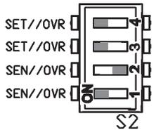
Override in Parallel with Setpoint: Common Ground Units
