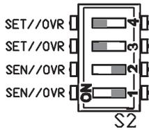
Override in Parallel with Setpoint: Differential Ground Units
