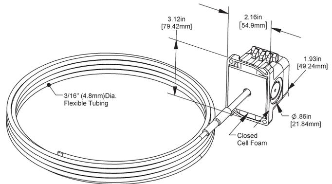
Fig 1: Submersible Averaging Unit with BAPI-Box Crossover Enclosure.
