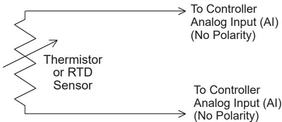
**Fig. 8:** 2-Wire Termination for Thermistor or RTDs
