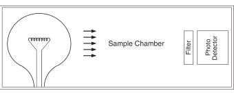
Figure 1: Single Channel CO<sub>2</sub> Sensor
