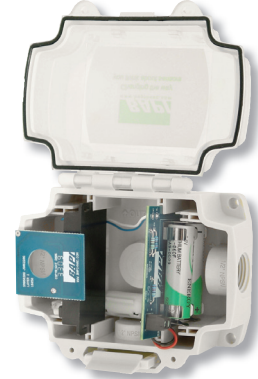
Wireless Analog or Digital Input Transmitter shown with the BAPI-Box open and closed
